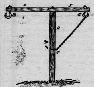
chain can turn easily; d is a chain running from c to e, which is a one-halfnch hook for hanging chain. On the other hookee, at other end of rod, b, hang the kettle. This arrangement allows the kettle to be swung off the fire easily at any moment, and without legs or anything under the kettle to interfere with building a fire. Such hanger is easy to make, but should be made of only good, strong material and put up substantial and firm.—E.
