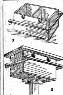
The box is divided in the center of its length by a partition, and a doorway is cut through one side of the box into each of the two compart-
