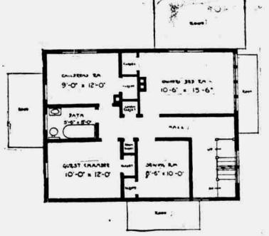
Frame two story dwelling, size 26x32 feet. Note the entry at front, also the large living room with large fireplace, plenty of light and living porch at the side. Stories: first 9 feet 4 inches; second 8 feet 6 inches. The interior is plaster stucco work, concrete foundation and slate roof. This house is very well lighted and planned. The projection of the cornice being so great gives the house a very cheering look.
