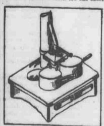
Stove Hood for Kitchen Use. of the kitchen and pass them up the chimney, instead of allowing them to permeate all parts of the house. His invention consists of a metallic hood, suspended above the stove and having an entrance directly into the pipe which leads to the chimney. Each cooking pot is provided with a cover
