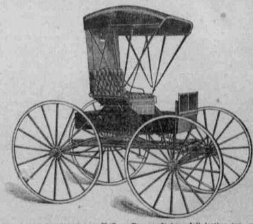
The above cut represents our Huffman Buggy. It has a full leather top, wood bows covered with leather, sliver plated joints, 14 double collar, steel axle, 14 steel tires, the best second girth, hickory gear and wheels, silver-tipped pole; body is 58 inches long, 30 inches wide, full circle, braced bottom and top; is a first-class job in every respect, and you can have the Buggy or \$150 in cash.
