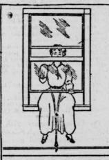
which a hook is attached. The cable washer straps the belt around his waist and takes his position on the window sill. The cable, as shown in the illustration, hangs inside and the hook can be anchored to some heavy piece of furniture or to another hool in the floor or surbase near the win dow. While this device was designed primarily for professional window cleaners, it will be found useful in private houses, especially where the servants are timid.
