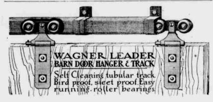
Our Leader Track in door hanger track construction. It is made of heavy stiff steel, will support any weight of door, is absolutely water proof, and owing to its self-cleaning feature, dust, dirt or any foreign matter cannot find lodgement, as it is carried out by the wheels being shaped to conform to the track.
