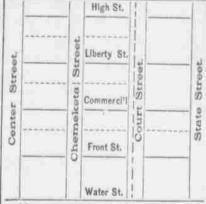
Above we give a diagram of our only sewer, running from the asylum and penitentiary through Court street to the river. The sewer is but 15 inches diameter, and serves the state buildings named, also the state house and is expected to be used by the four tiers of blocks lying between Ferry and Center streets. The dotted lines represent the main sewer and laterals through Court street and the alley ways.
