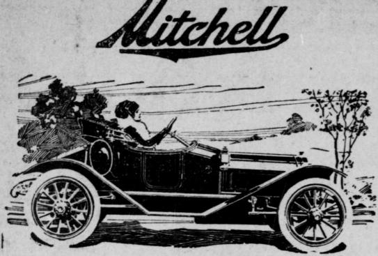
The above Roadster has 100 inch wheel base, 32x3 1-2 tires, of Olmito were visitors in the city Standard Universal Rims, cone clutch, 30 horsepower long stroke motor, four cylinder, Ssplitdorf Dual System Ignition, selective type transmission, three speeds forward and reverse, full floating rear axle.
