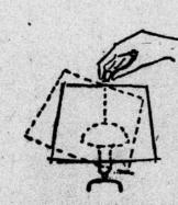
The Levelizer: A patented device (with rounded surfaces instead of the usual flat surfaces on the shade and its support) allows the shade to automatically level itself.
