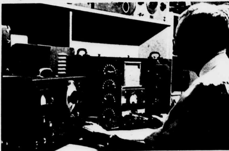
Earl D. Ball, electronics engineer, calibrates a signal generator (left), part of the equipment used by FCC field men. *Star Staff Photos by Elwood Baker.*
