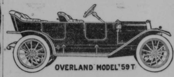
Wheelbase 106 inches: motor 4x4 1-2; horsepower 20; Splitdorf magneto: transmission selective, 3 spee ds and reverse; F. and S. ball bearings; tires 32x3 1-2 Q. D.; 3 oil la mps, 2 gas lamps and generator Complete set of tools.
