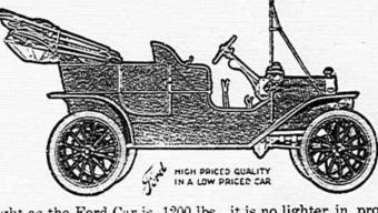
Light as the Ford Car is, 1200 lbs., it is no lighter in proportion than a passenger engine of the accepted highest type. The 5000 H. P. Pacific type locomotive used on the Pennsylvania Lines West weighs 53.8 lbs. per horse power. The Model "7" weighs 53.3 lbs. per horse power. Each is designed by an engi neering expert for passenger service. On the other hand, the average freight engine, as well as a large proportion of autome biles, weighs from 85 to 110 lbs. per horse power. Note the dif
