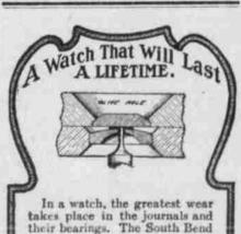
takes place in the journals and their bearings. The South Bend Watch has journals - called pivots-made of the finest quality of steel, tempered by a special process and brought to an absolutely perfect finish. Their bearings are the finest imported jewels, carefully select-ed and polished with specially prepared diamond powder. They are practically proof against
