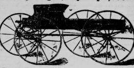
This makes the most complete, low down and light de-livery wagon on the market. Equipped with our adjustable foot board and high riser seat. Double bent shafts, heavily ironed. Length, 7 feet; 34 inches wide outside. We make this wagon in any size to order, and let-tered in gold leaf or any style desired.
