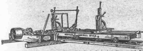
It is the lightest running, easiest handled, fastest cutter, most durable and satisfactory Saw Mill on the market. No other mill in the world has so many time and labor saving inventions all in one, at such a low price. It has steel head blocks, bottom and top dogs, automatic offset of the log when gigged back, spring receder, steel lined carriage, taper knees, wire cable drive, etc.
