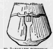
NO. 2-NAILLESS HORSESHOE. pressed, and there is abundant room for the expansion of the foot in every direction, assuming expansion to take place at all To remove the shoe it is only necessary to reverse the previous process -release the loop of the band from the front pillar, and the shoe at once come
